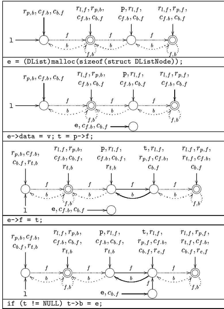
Table XVII: The abstract interpretation of the `splice` procedure applied to a doubly linked list whose head is pointed to by `1`. Variable `p` points to some element in the list beyond the second element, and the tail of `p` is assumed to be non-NULL. For brevity, node names are not shown, and  $r_{z,f}(v)$  and  $r_{z,b}(v)$  are omitted when  $v$  is directly pointed to by variable  $z$ .
