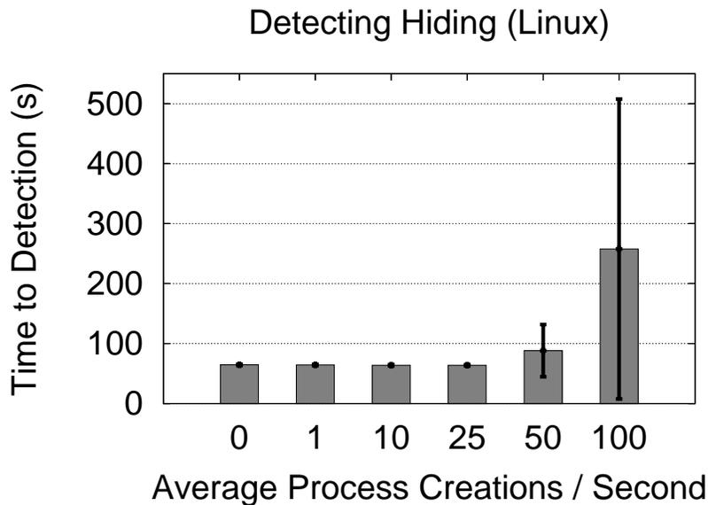
Figure 6.6: **Time to Detection.** The figure shows how the time to detect a hidden process varies for Linux as process creation and exit activity increases from 0 processes/second to 100 processes/second. The values shown are an average of 10 trials. Error bars show the standard deviation of detection time.
