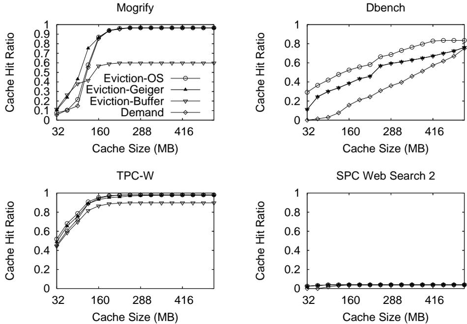
Figure 5.14: **Secondary Cache Hit Ratio.** The figure compares the cache hit ratio in a secondary storage cache for various workloads when demand placement (*Demand*), eviction placement based on inferred evictions (*Eviction-Buffer* and *Eviction-Geiger*), and eviction placement based on actual evictions (*Eviction-OS*) is used. Experiments are performed using cache sizes from 32 MB to 512 MB.
