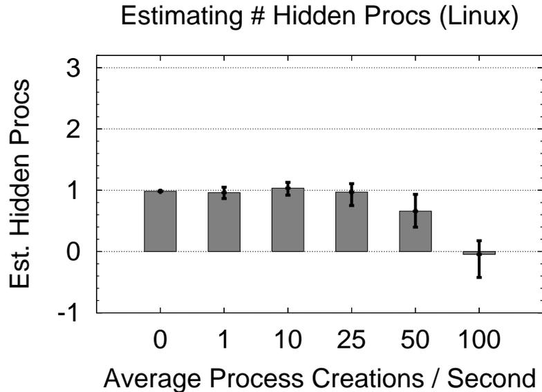
Figure 6.7: **Estimating the Number of Hidden Process.** The figure shows how the estimate of the number of hidden processes obtained from the detection phase varies for Linux as process creation and exit activity increases from 0 processes/second to 100 processes/second when a single process has been hidden. The values shown are an average of 10 trials. Error bars show the minimum and maximum hidden process estimate observed.
