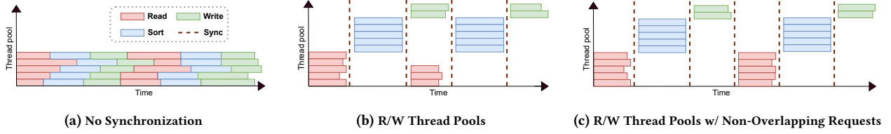
Figure 2: Three different concurrency mechanisms. To maximize BRAID device bandwidth, WiscSort prefers 2c model (interference aware, thread-pool controller) over 2b (thread-pool controller) and 2a (interference unaware). In all three models, the sort pools are the same size; the size of read and write pools may differ for (b) and (c).
