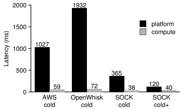
Figure 21. AWS Lambda and OpenWhisk. Platform and compute costs are shown for cold requests to an image-resizing lambda. S3 latencies are excluded to minimize noise.
