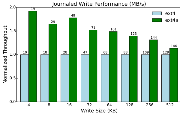
Figure 4: Data journaling write throughput with ANViL-optimized ext4a compared to unmodified ext4. Each bar is labeled with absolute write bandwidth.
