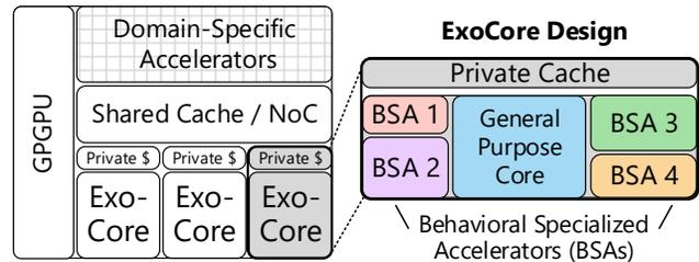
Figure 1: ExoCore-Enabled Heterogeneous System
