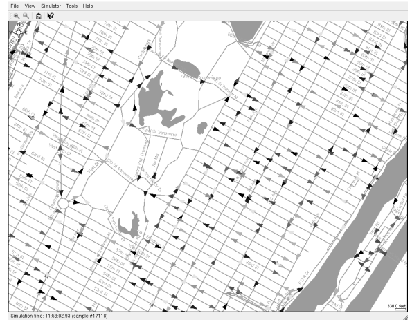
Fig. 4. TRAC Simulator with 650 vehicles driving around in Manhattan, NY, USA
