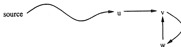
Figure 9.1. An example to show how the presence of cycles complicates determining if the deletion of an edge u \rightarrow v leaves vertex v unreachable. It is not sufficient to check if v has some predecessor marked reachable. We need to determine if v has some predecessor that is marked reachable and is not dominated by v . All vertices in the above example are marked reachable to begin with.
