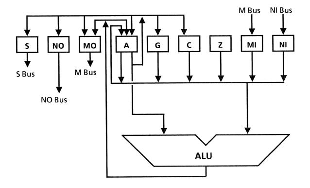
In the typical case, the ALU instructions take the value of the accumulator as one operand, the value of a memory location (held in the MIreg) as the second operand, apply a given operation, and return the result to the accumulator. Alternatively, the ZERO pseudo register may be used as an operand instead of memory, and the result of the operation may go to memory, rather than to the Areg. In all cases, the complemented values of the source registers may be used as operands.
