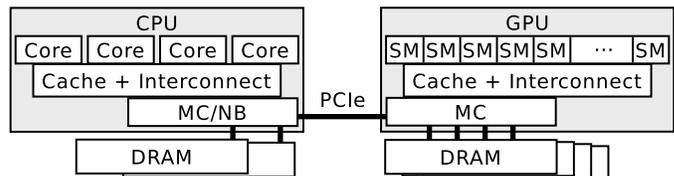
Fig. 1. Discrete GPU system with separate CPU and GPU chips.
