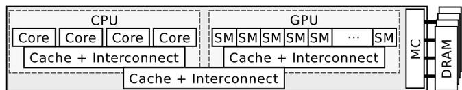
Fig. 2. Heterogeneous processor with integrated GPU on a single chip.
