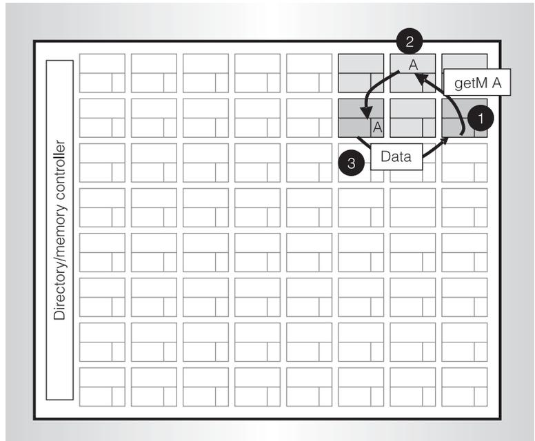
Figure 4. First level of coherence in a virtual hierarchy enables fast and isolated intra-VM coherence: A processor issues a request to the dynamic home tile that is local to the VM (1). A directory tag is found and the request redirects to the owning tile with dirty data (2). The owner responds to the requester (3).
