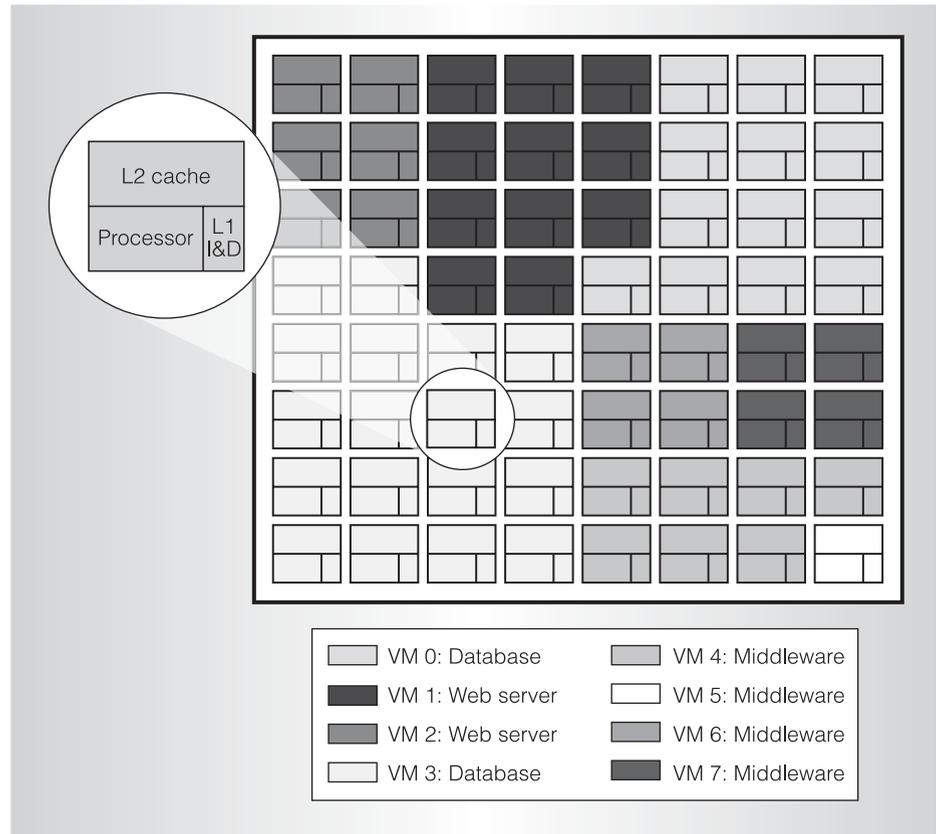
Figure 1. Tiled chip multiprocessors (CMP) running consolidated servers.
