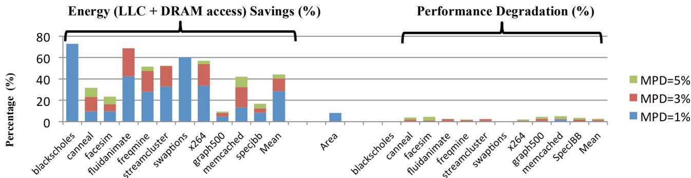
Figure 5. Energy/area savings and performance degradation with FreshCache.
