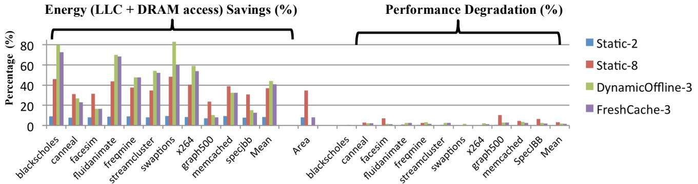
Figure 6. Energy savings and performance degradation for dynamic dataless ways under hardware control.
