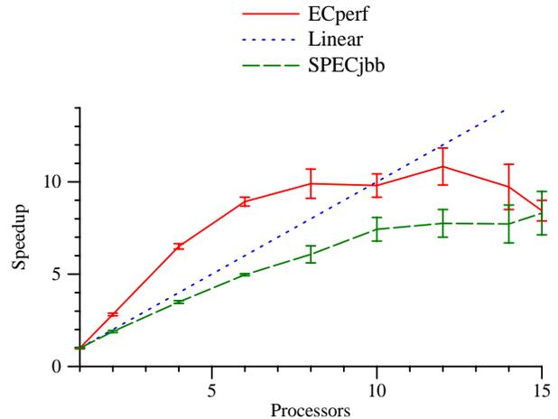
Figure 4: Throughput Scaling on a Sun E6000
