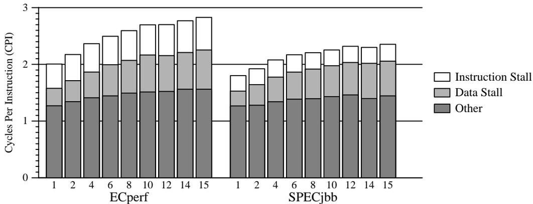
Figure 6: CPI Breakdown vs. Number of Processors
