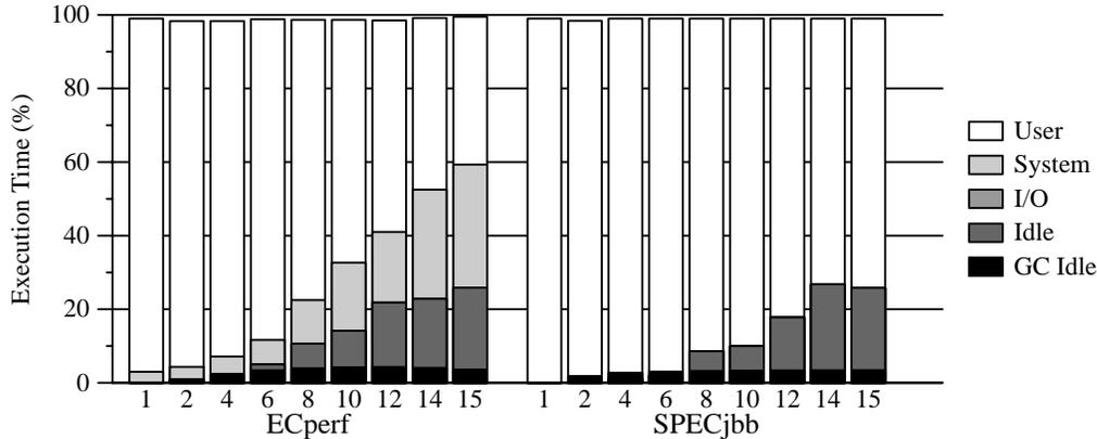
Figure 5: Execution Mode Breakdown vs. Number of Processors
