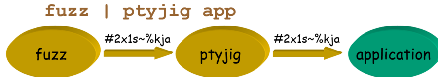
Figure 2: The Simplest Forms of Fuzz Testing: Piping Random Input to a Program
