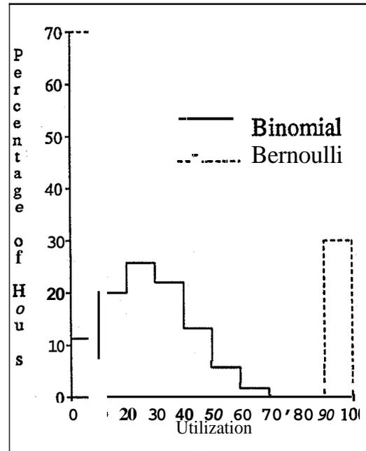
Figure 3.5: Bernoulli and Binomial Probability Density Functions
