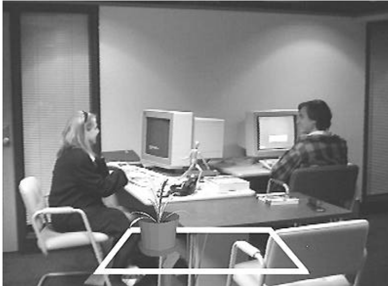
Figure 8.7: A 3D image overlaid on top of a corresponding real image. Our goal is to place the virtual plant on the real table. In each image, there is a table (denoted by the white rectangle for the graphics image). Initially, the images do not correspond because the virtual camera is not in the same place as the camera used to create the real image.
