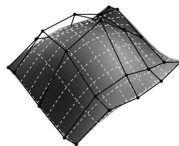
Figure 1-24. Moving the control points of a patch changes the shape of the patch.
