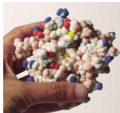
Figure 4. Rapid prototyping methods are being used to create physical models of large molecules. This model of chymotrypsin (notice the deep, dark specificity pocket) was created by using machinery from Z-Corporation. The machinery lays down thin layers of gypsum powder and sprays on colored glue with an ink-jet printer, building the model up layer-by-layer from bottom to top. The hand-sized model allows direct, tactile exploration of the protein structure.
