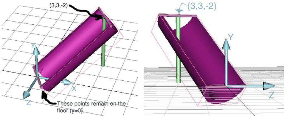
Provide a matrix that transforms the initial half-pipe to the final configuration.
