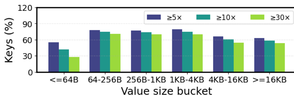
Figure 4.4: Intra-key reuse-distance spread in Meta KV traces. Bars show the fraction of keys in each value-size bucket whose reuse-distance interquartile range ( p_{75}/p_{25} ) exceeds 5\times , 10\times , or 30\times . A larger spread indicates frequent transitions between hot and cold phases for the same key.
