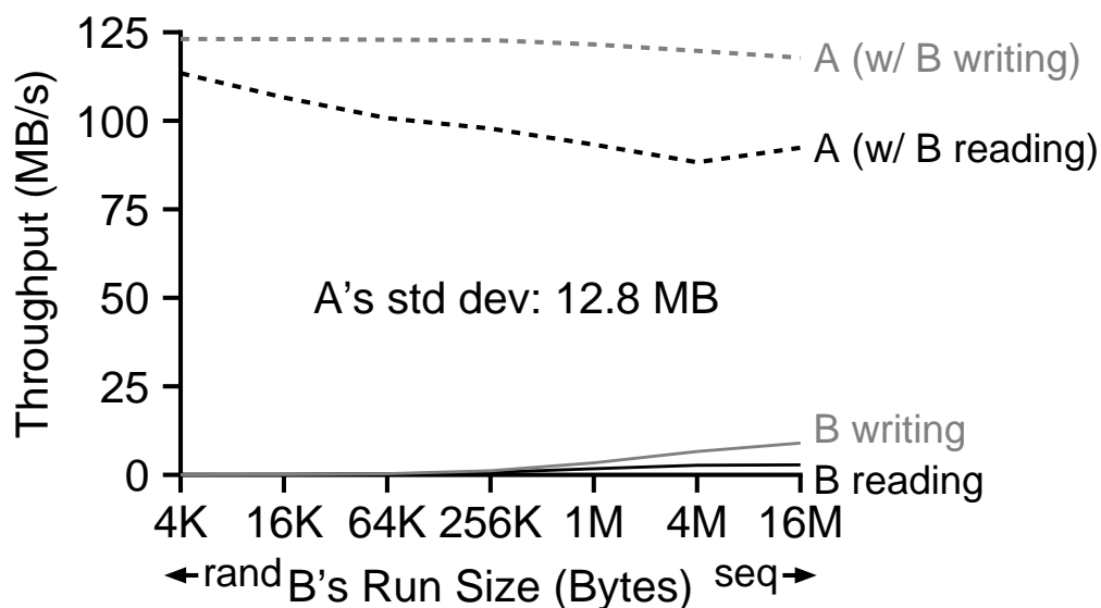
Figure 2.18: Isolation: Split-Token with XFS. This is the same as Figure 2.7 and Figure 2.16, but for XFS running with our Split implementation of token bucket.
