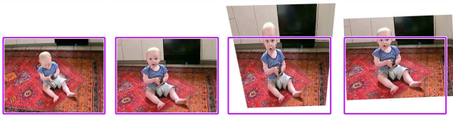
Figure 4: The projective transformation can stabilize the carpet between two frames (left 2 images), but stretches objects out of this plane (middle right). The rightmost image shows the similarity transform closest to the projective homography.
