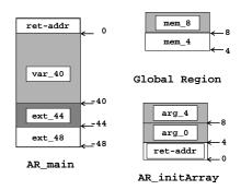
Fig. 7. Layout of the memory-regions for the program in Ex. 3.2. (LocalGuard and FormalGuard are not shown.)
