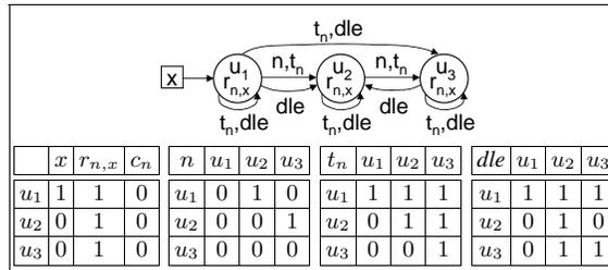
**Fig. 2.** A logical structure  $S_2$  that represents the store shown in Fig. 1 in graphical and tabular forms.
