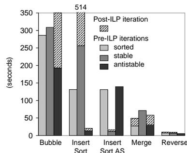
**Fig. 13.** Execution times. For each program, the three bars represent the sorted, stable, and antistable queries. In cases where subformula-based refinement failed, the upper portion of the bars shows the cost of the last iteration of the analysis (on both the DSC and the program) together with the ILP cost.
