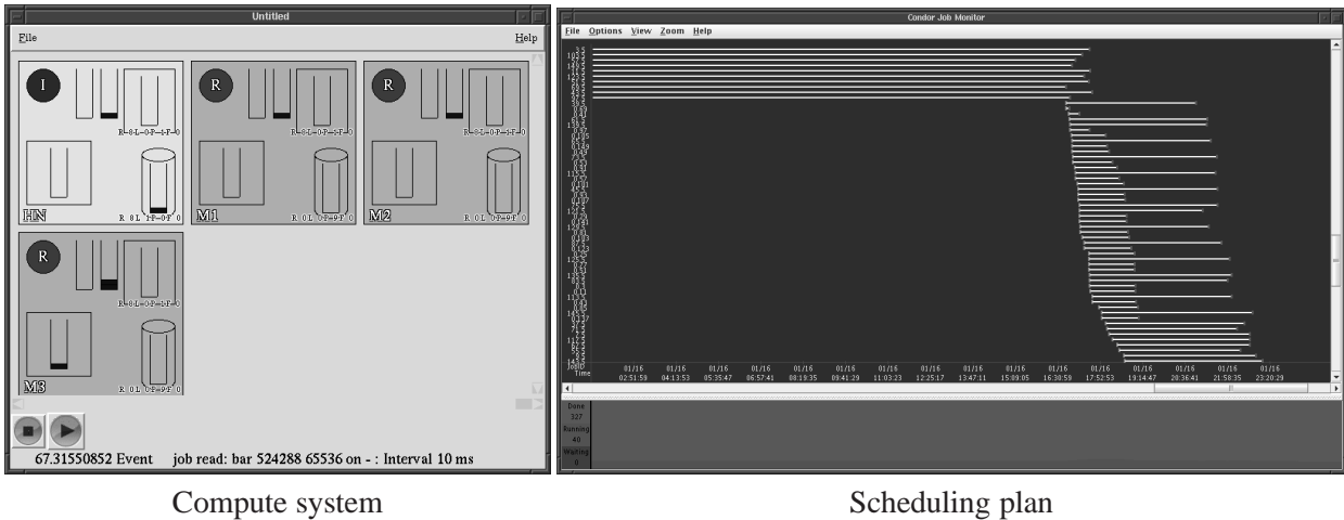
Figure A.2: Validating Functional Correctness of the Compute System and the Scheduler. The illustration on the left shows a representation of the compute system including the disks, buffer caches, and network queues for each machine. On the right is a visualization of the execution schedule for a workload with inter-job dependencies.
