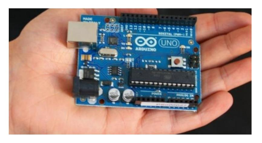
Atmel chip, 14 digital input/output pins, 6 analog inputs, a 16 MHz crystal oscillator, a USB connection, 32KB Flash, 2KB SRAM
