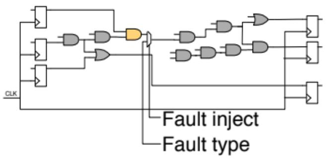
Add fault injection logic
