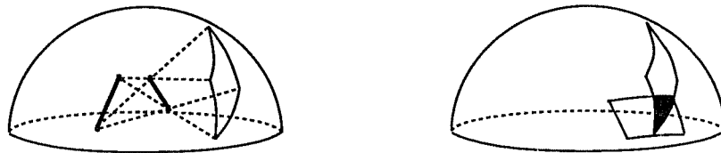
Figure 7. (a) A T-junction will occur between the two edges from any viewpoint within the patch on the view sphere. (b) Two T-junctions co-occur in the image plane when the viewpoint is in the intersection of the patches for each T-junction on the view sphere.
