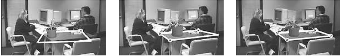
Figure 8.8: The synthetic and real images are registered by successively dragging the corners of the table to their corresponding positions in the image.
