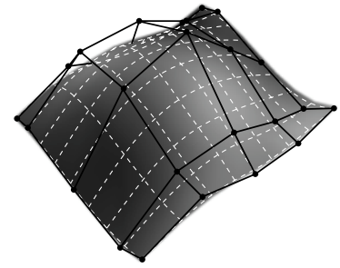
Figure 1-24. Moving the control points of a patch changes the shape of the patch.
