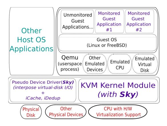
Sky is 7.8 KLOC of new code added to 43.6 KLOC of KVM Pseudo device driver in the host (3.8 KLOC of source code) Bcache (10% new code), Dmdedup (14.5% new code)
