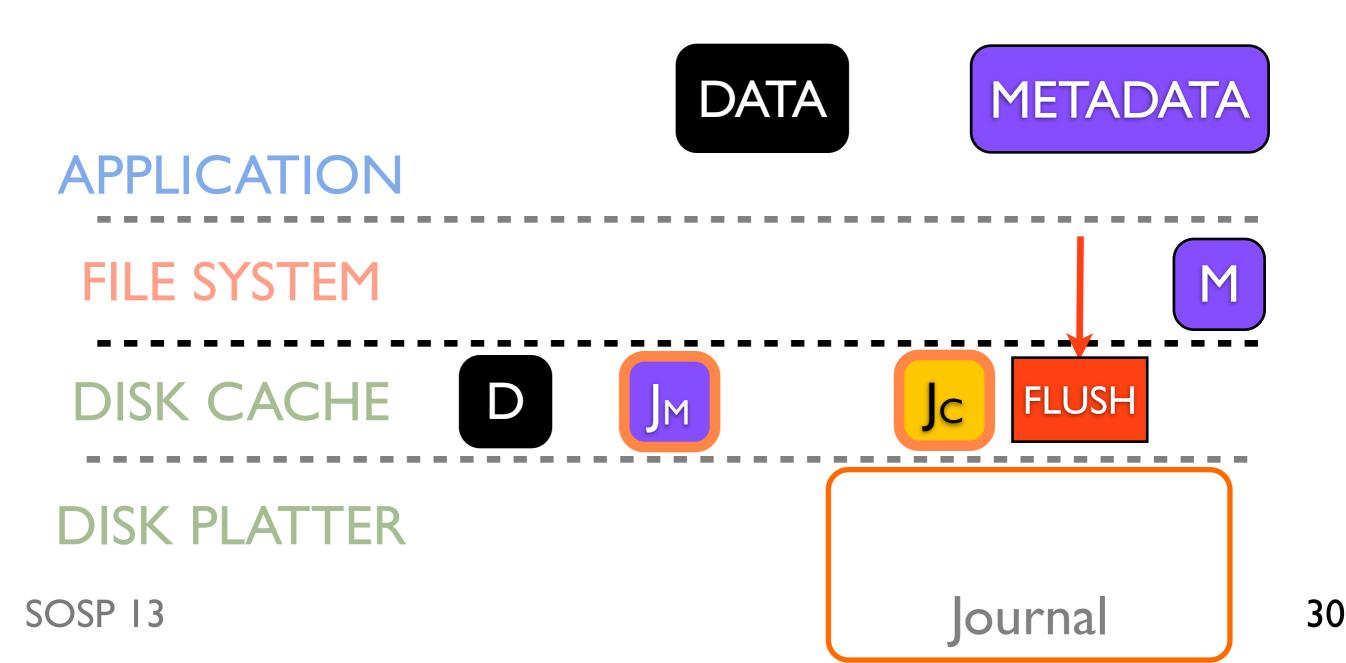
Checksums and Delayed Writes handle reordering from removing flushes
