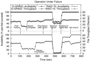
Figure 9: **Availability Profile.** The figure shows the operation of D-GRAID Level 1 and RAID 10 under failures. The 3 GB array consists of 4 data disks and 1 hot spare. After the first failure, data is reconstructed onto the hot spare, D-GRAID recovering much faster than RAID 10. When two more failures occur, RAID 10 loses almost all files, while D-GRAID continues to serve 50% of its files. The workload consists of read-modify-writes of 32 KB files randomly picked from a 1.3 GB working set.
