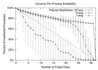
Figure 3: **Dynamic Data Availability.** The figure plots the percent of processes that run unaffected under disk failure from one busy hour from the HP trace. The degree of namespace replication is set aggressively to 32. Each line varies the amount of replication for "popular" directories; 1-way implies that those directories are not replicated, whereas 8-way and 32-way show what happens with a modest and extreme amount of replication. Means and deviations of 30 trials are shown.
