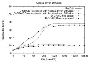
Figure 7: Access-driven Diffusion. The figure presents the performance of D-GRAID Level 0 and standard RAID-0 under a sequential workload. In each experiment, a number of files of size x are read sequentially, with the total volume of data fixed at 64 MB. D-GRAID performs better for smaller files due to better physical block layout.
