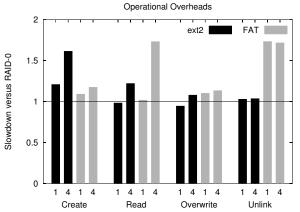
Figure 6: **Time Overheads.** The figure plots the time overheads observed on D-GRAID Level 0 versus RAID Level 0 across a series of microbenchmarks. The tests are run on 1 and 4 disk systems. In each experiment, 3000 operations were enacted (e.g., 3000 file creations), with each operation on a 64 KB file.
