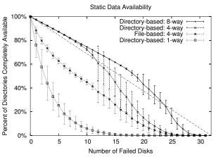
Figure 2: Static Data Availability. The percent of entire directories available is shown under increasing disk failures. The simulated system consists of 32 disks, and is loaded with the 250 GB from the HP trace. Two different strategies for semantic grouping are shown: file-based and directory-based. Each line varies the level of replication of namespace meta-data. Each point shows average and deviation across 30 trials, where each trial randomly varies which disks fail.
